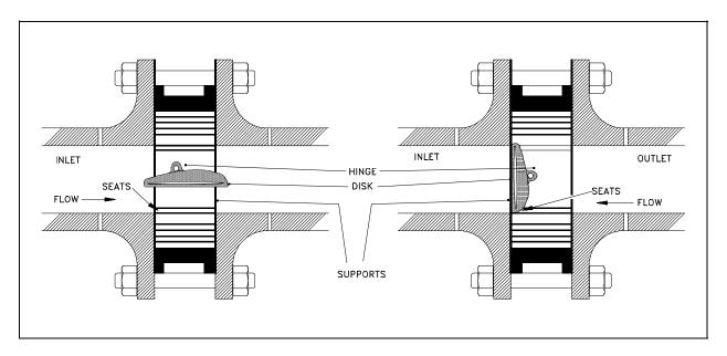
Figure 23 Operation of Tilting Disk Check Valve
