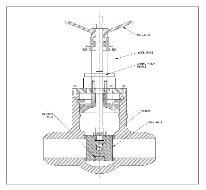
Figure 8 Parallel Disk Gate Valve
