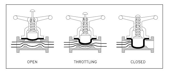
Figure 14 Straight Through Diaphragm Valve
