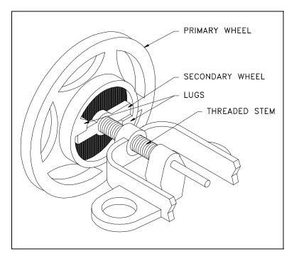
Figure 31 Hammer Handwheel
