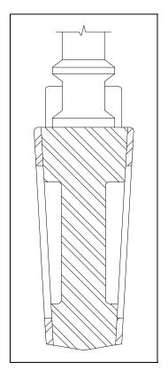
Figure 5 Solid Wedge Gate Valve
