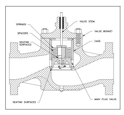
Figure 25 Piston Check Valve
