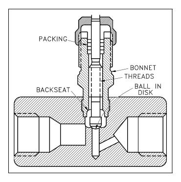
Figure 21 Bar-Stock Instrument Valve
