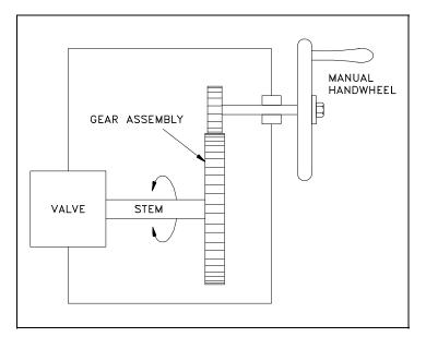
Figure 32 Manual Gear Head
