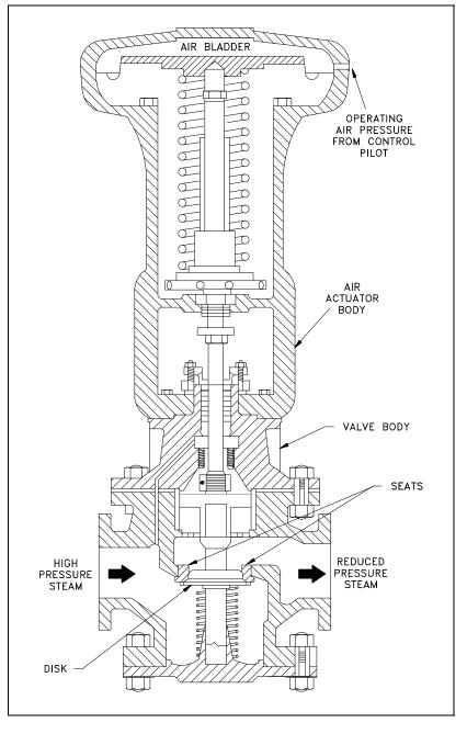
Figure 34 Pneumatic Actuator
