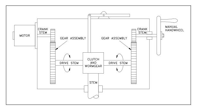
Figure 33 Electric Motor Actuator
