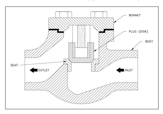
Figure 24 Lift Check Valve
