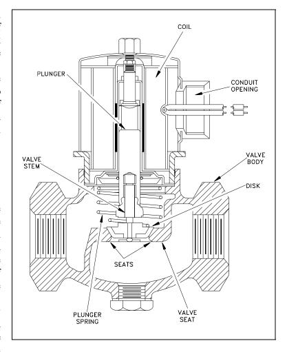
Figure 35 Solenoid Actuated Valve
