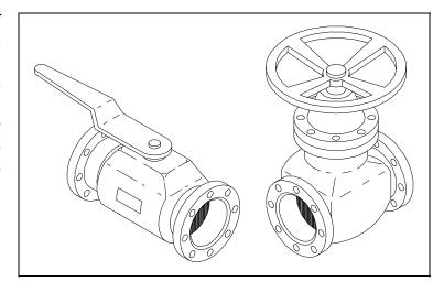
Figure 30 Fixed Handwheel
