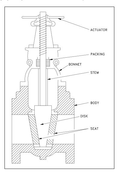
Figure 1 Basic Parts of a Valve
