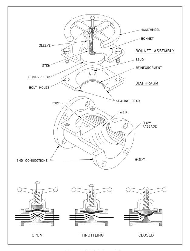
Figure 15 Weir Diaphragm Valve
