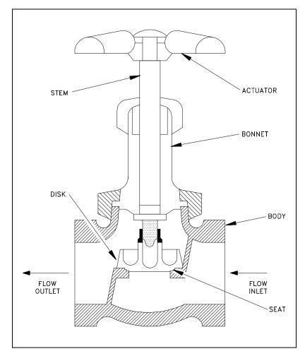
Figure 27 Stop Check Valve
